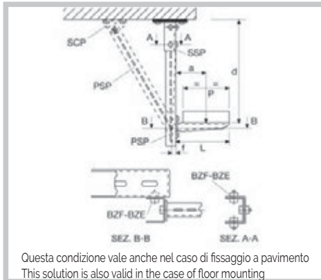
SOSPENSIONE CON PROFILATO - PSP CEILING SUPPORT WITH PSP U-SECTION
