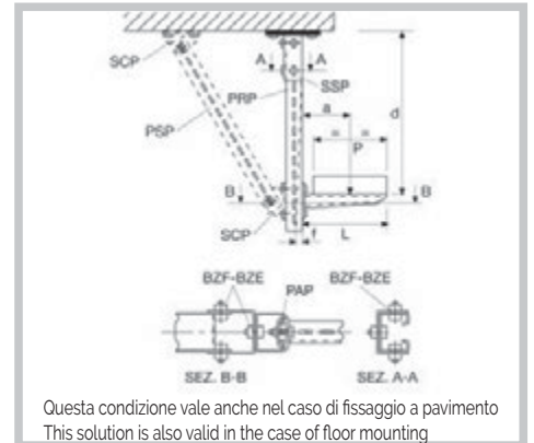
SOSPENSIONE CON PROFILATO - PRP CEILING SUPPORT WITH PRP U-SECTION
